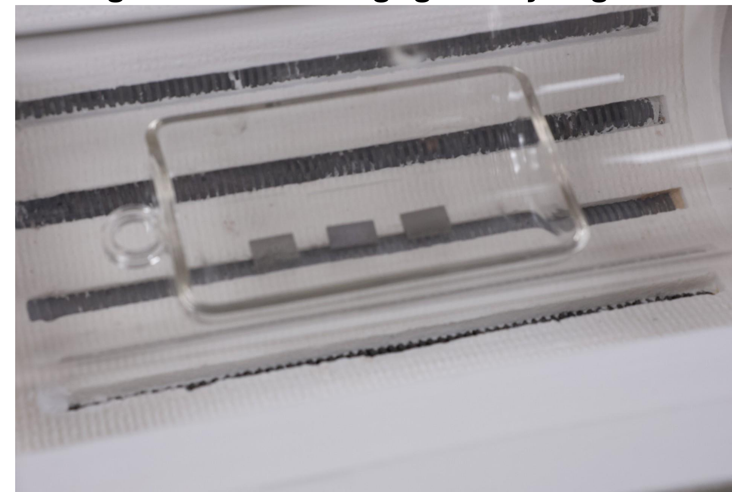
Fig 3. Materials being aged in hydrogen
